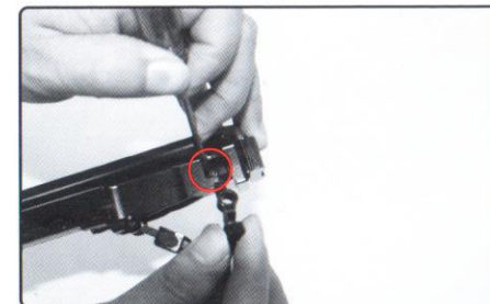
組裝槍機釋放鈕時，請用一字起子先將覆進簧桿後推固定，以便槍機釋放鈕裝入 While installing the bolt release lever, push the recoil spring first with a flat blade screwdriver and put in the bolt release lever.
