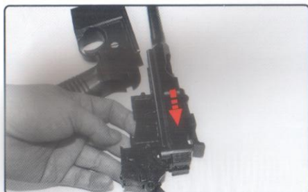
即可上下槍身分離 This enables the upper barrel to be separated from the lower barrel.
