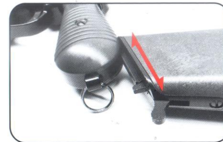
組裝或卸下時請將槍托卡溝槽順握把之槍托卡溝推入或拉出 The stock doubled as a case or holster, and attached to a slot cut in the grip frame.
